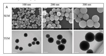
Figure II. Morphological characterization and structure diagram of TiO<sub>2</sub> PEG nanoparticles of different sizes. TiO<sub>2</sub>-PEG nanoparticles 100, 200, and 300 nm in size were characterized by SEM (upper panels) and TEM (lower panels). Both SEM and TEM images showed that the nanoparticles were spherical and uniform. The characterization of TiO<sub>2</sub>PEG NPs confirmed the enhancement effect of PEG-glycation on the dispersity and uniformity of TiO<sub>2</sub> NPs [23].
